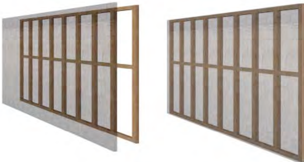
The 'secretion lining' provides a shell for wooden framework.
